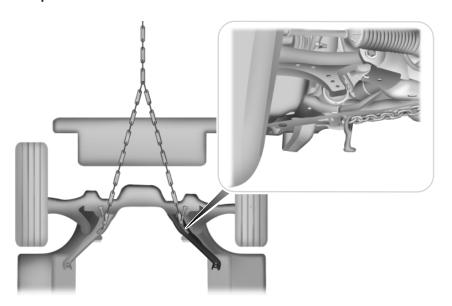
When towing the vehicle, make sure that you use two mini J hooks and attach them to the crossmember oblong holes as shown to winch the vehicle onto the flatbed. The T-hook slot should be used to tie-down the vehicle to the wrecker. Other methods may damage the vehicle.
