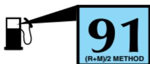
rating of 91 or higher for optimum performance. The use of gasolines with lower octane ratings may degrade performance. We do not recommend the use of gasolines labeled as “Premium” in high altitude areas that are sold with octane ratings of less than 91.
