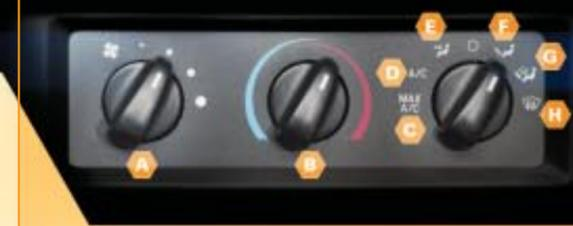
**A FAN SPEED CONTROL** Rotate the knob to adjust the volume of air circulated in the vehicle.
